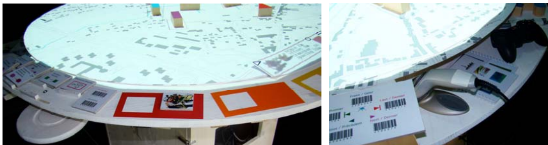
Figure 13 – Configuration area with viewpoint wheel, command cards, RFID color zones, barcode tray, barcode reader and remote control
