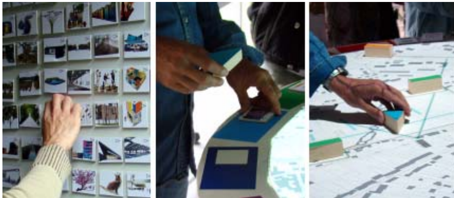
Figure 16 - Re-designed chain of actions to add an object to the scene: Selecting content (a), selecting a token, assigning the content (b) and placing the token (c).
